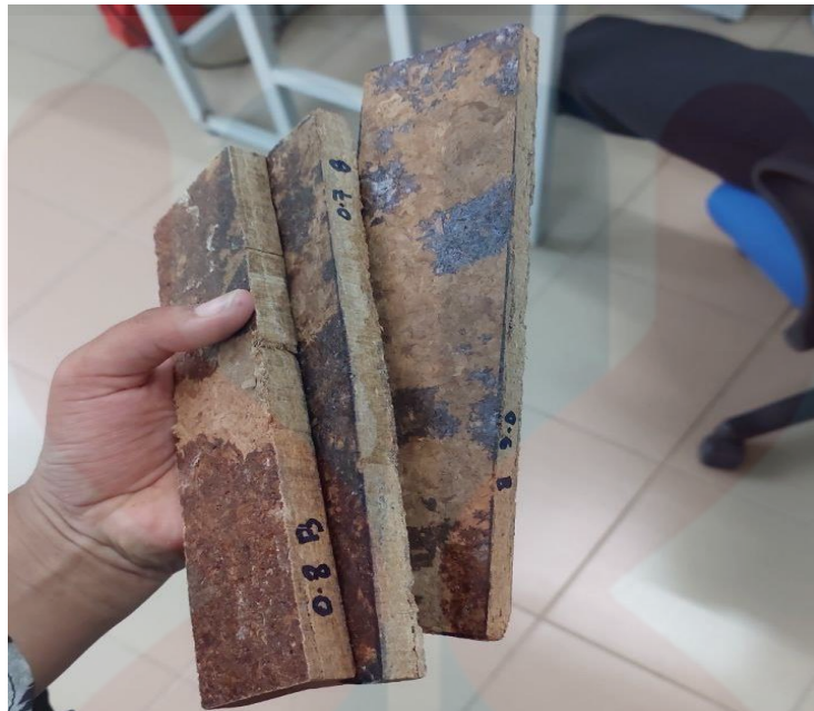
Figure 24: Particle board sample for bending test
