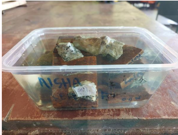
Figure 20: Particle board sample was immersed in water for water absorption for 1 hour, 2 hours and 24 hours.
