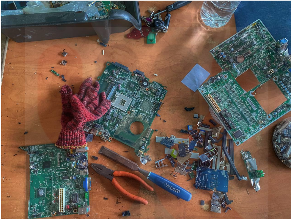
Figure 3.3: the component containing gold has been separated from the circuit boards or CPUs
