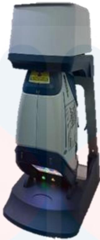
Figure 2.2: Example of X-ray fluorescence machine
