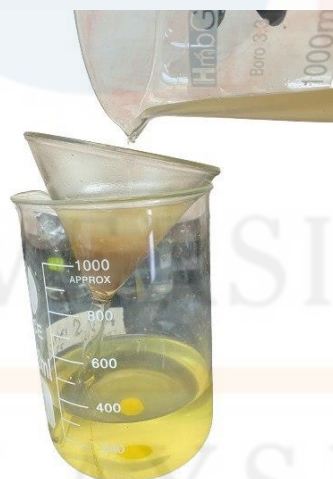
Figure 3.5: gold filtered using cotton and funnel
