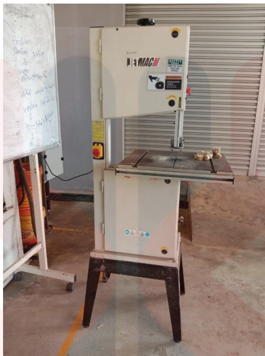
Figure A.3: 14" Wood band saw used to cut bamboo into small sizes
