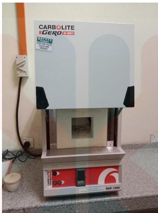
Figure A.5: Furnace 1500°C (Carbolite Gero Sheffield, United Kingdom) for activation bamboo
