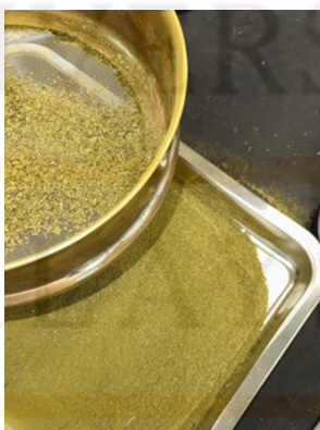
Sieving using steel sieve 0.5mm
