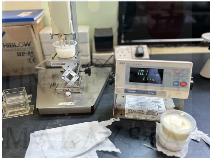
Figure 4. Vibro viscometer used to calculate viscosity of cream
