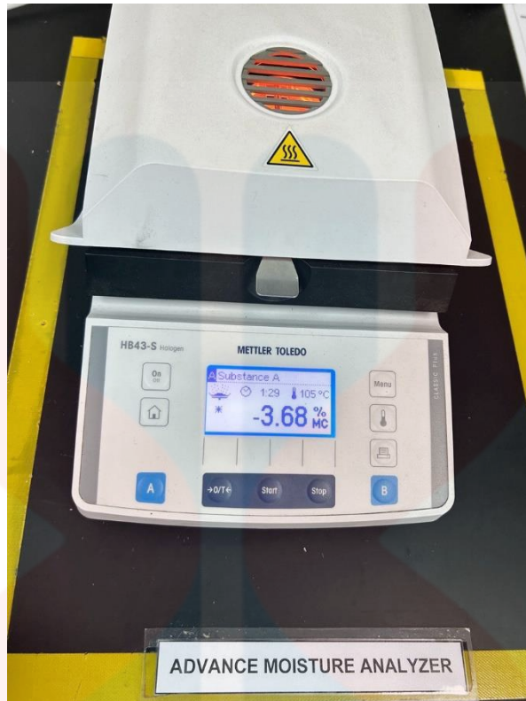
Figure 3. Advance moisture analyzer that used to calculate moisture content in cream
