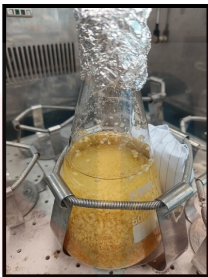
Figure 3.2: Pre-treatment process of dry corncob using 1.4% \text{NaClO}_2
