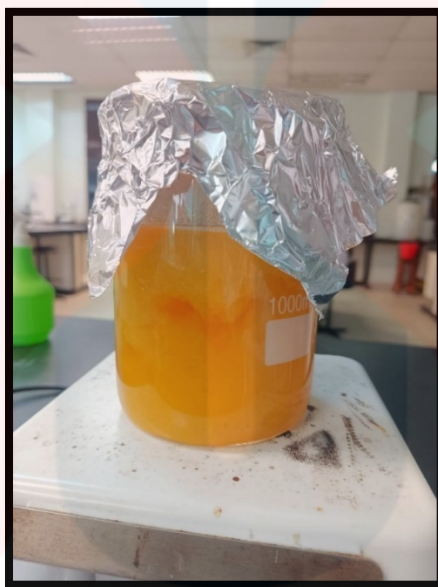
Figure 3.4: Extraction of cellulose using 5% KOH
