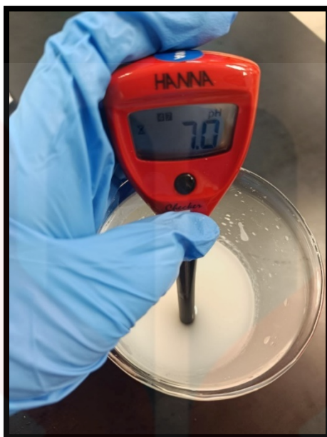
Figure 3.5: KOH-treated sample that has been washed with distilled water
