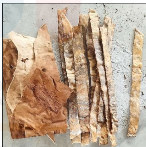
Figure A.4: Cutting the hides by using angle grinder, band saw machine
