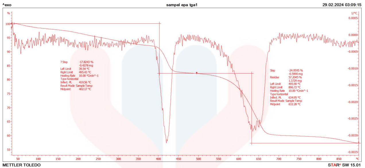
Figure 4.3 : TGA analysis for EPA catalyst
