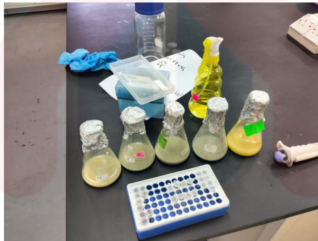
Figure A.2: the ore sample turns grey yellow colour after bioleaching for 20 days
