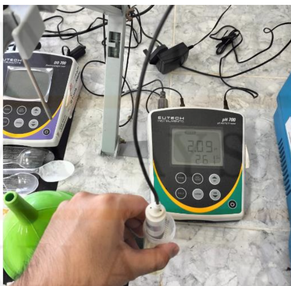
Figure A.6: culture medium maintains at 2.09 pH value after bioleaching
