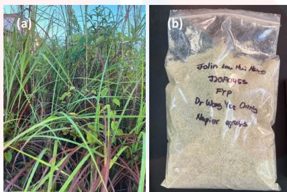
Figure 3. 1: (a) Napier Grass found in Taman Pinggiran, UMK Jeli Campus; (b) Napier Grass Powder After Drying and Grinding
