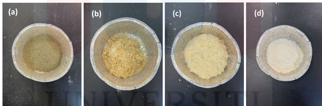
Figure 4. 1: Photographs image: (a) raw Napier grass (b) alkaline-treated sample (c, d) Bleached sample and (d) extracted cellulose sample.
