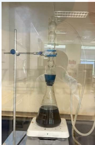
Figure 3. 2: Alkaline treatment under reflux system.
