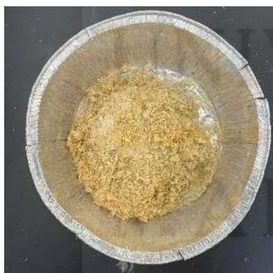
Post-alkaline treatment, the sample colour turned slightly brighter yellowish.
