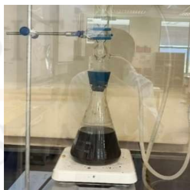
The grass powder underwent alkaline treatment with reflux for 3 hours.
