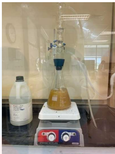
Figure 3. 3: Bleaching treatment under reflux system.
