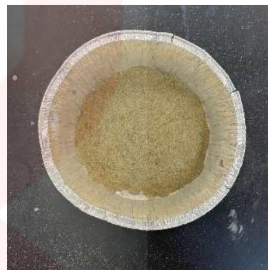
The grass was dried at 65°C for 24 hours and ground into a fine powder.
