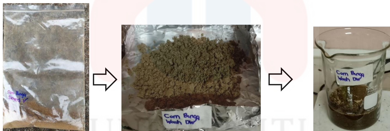
Figure 4. 5: The corn tassel changes colour from brown to dark brown after alkaline treatment with toluene-ethanol mixture
