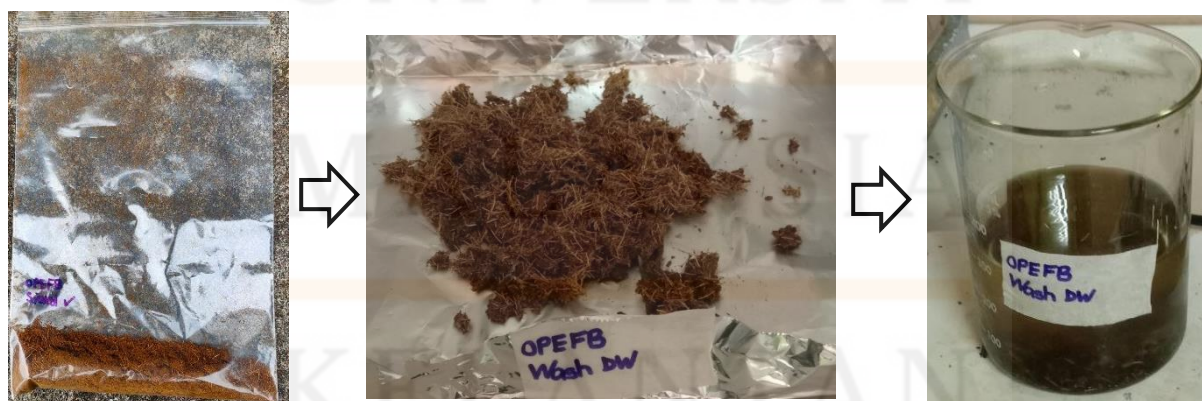
Figure 4. 7: The oil palm empty fruit bunch changes colour from brown to dark brown after alkaline treatment with toluene-ethanol mixture
