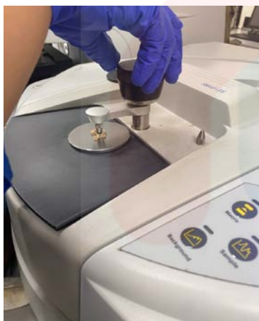
Testing FTIR of soap sample 2
