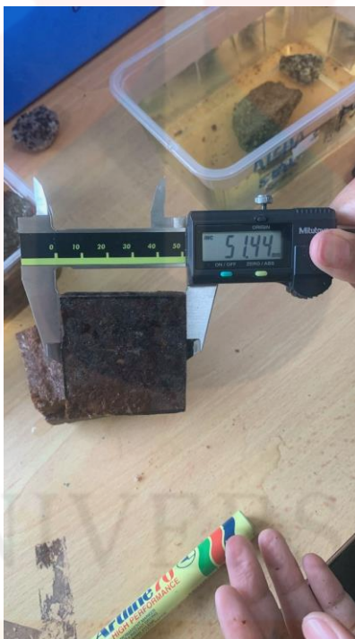
Figure 19: Measure the thickness of particleboards
