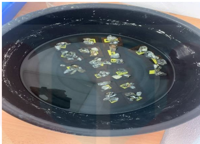
Figure 18: Water absorption and thickness swelling process
