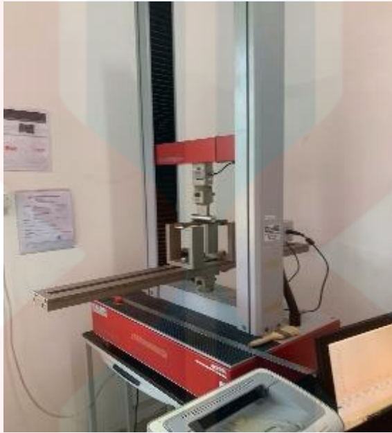
Figure 16: Machine of bending test
