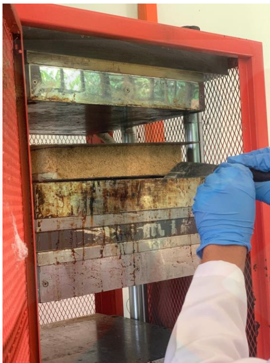
Figure 14: manufacturing the particlebords
