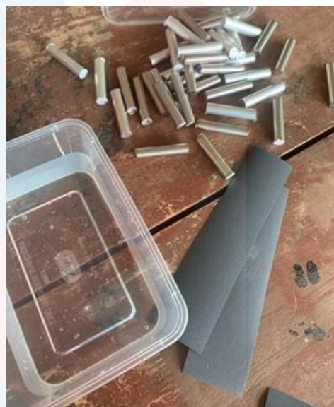
Apparatus and preparation of electrode for electrocoagulation process
