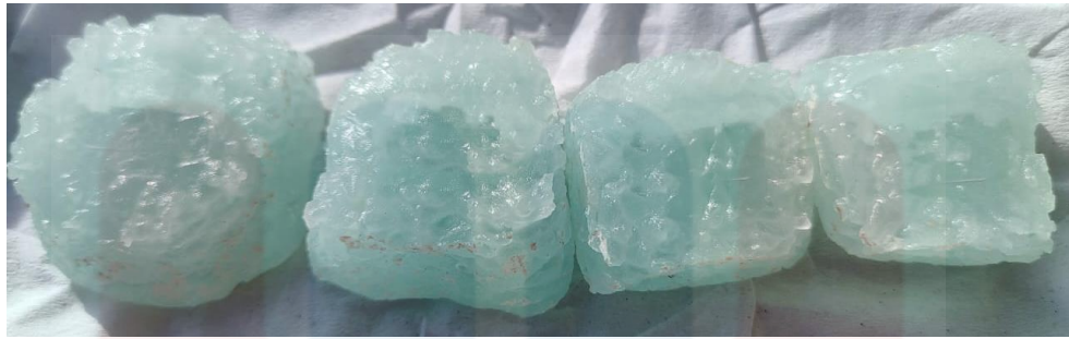
Figure 4.17: The production of glass bricks by using cullet of waste glass with 950 °C and 8 hours exposure time
