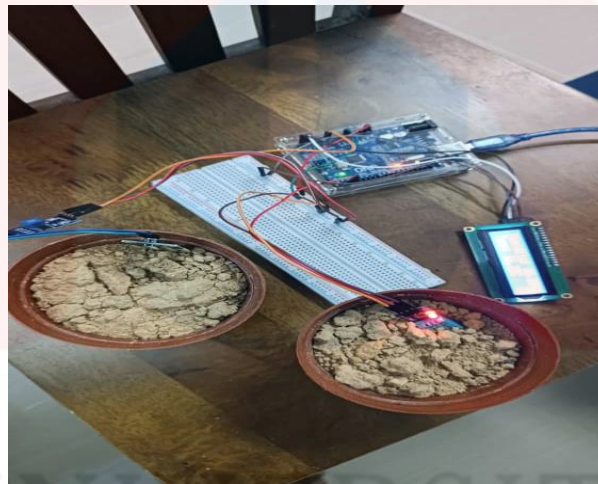
Figure 4. 5: Device connection of sensors during soil testing
