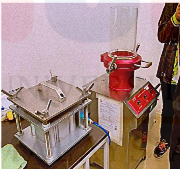
Figure 3.3.3.1: Hand sheet machine and presser machine.
