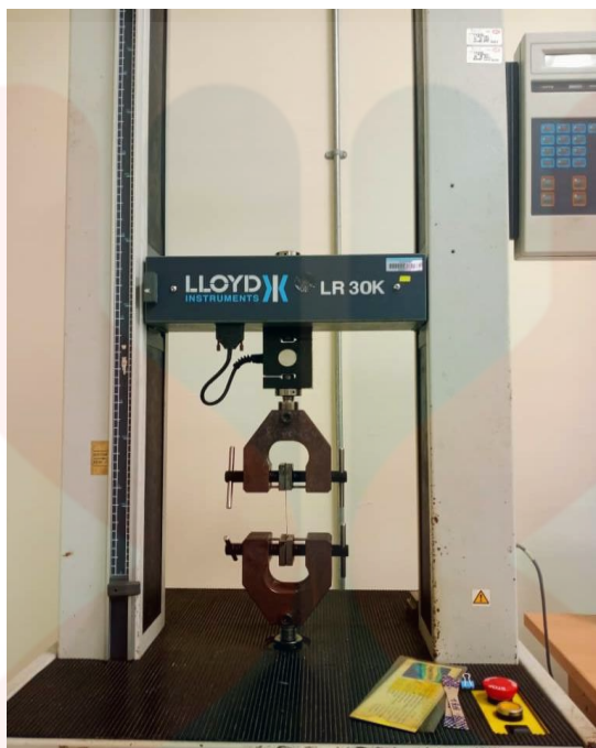
Figure 3.3.7.1: Uniform testing machine for tensile strength and tear determination.
