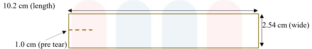
Figure 3.3.8.1: Illustration tear paper film.
