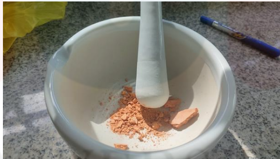
Figure 3.2: The defect Singgora tiles were crushed.
