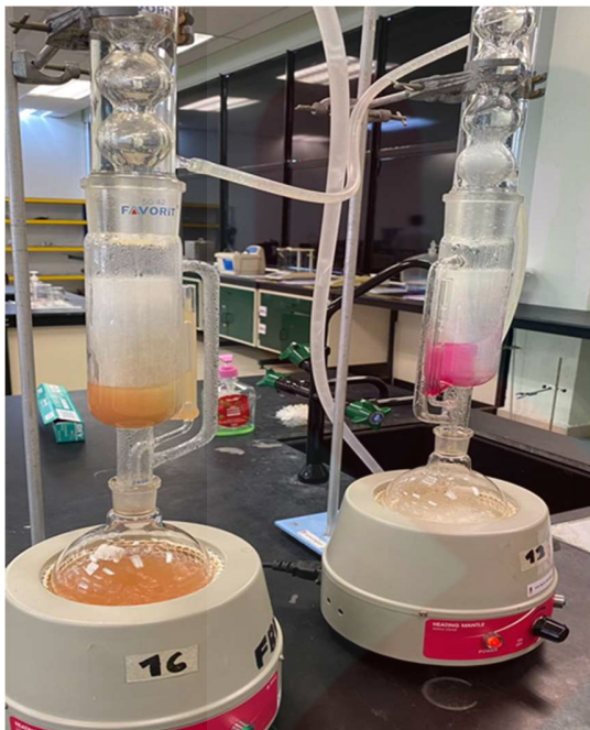
Figure B.3: Preparation of dye extraction of ethanol and deionized water using soxhlet.
