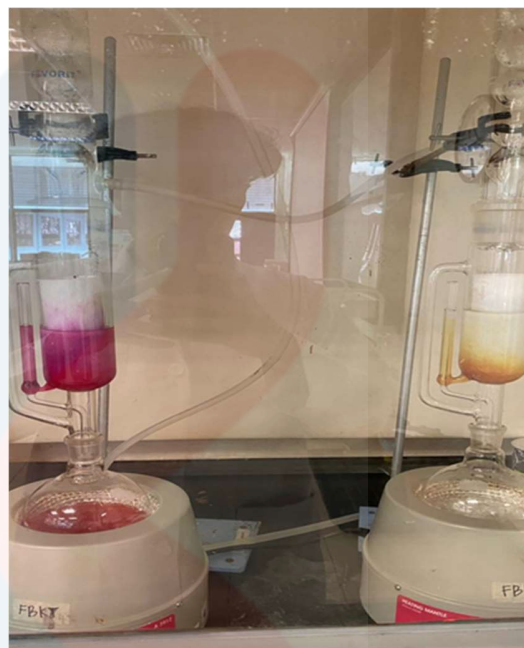
Figure B.3: Preparation of dye extraction of ethanol and deionized water using soxhlet.
