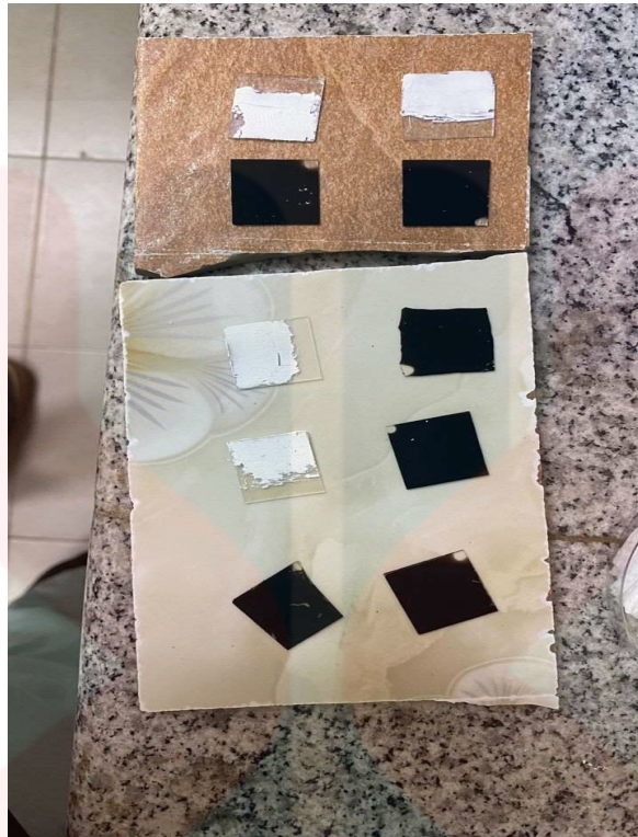
Figure B.5: TiO 2 paste was deposited on the ITO glass and activated carbon was applied on the remaining substrates using the doctor blade method.
