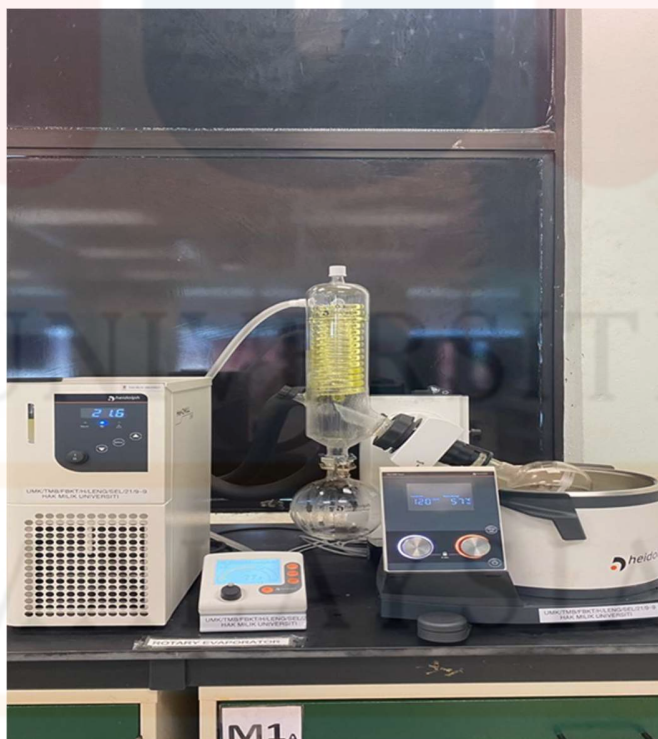
Figure B.4: Preparation of dye extraction of samples using rotary evaporator.
