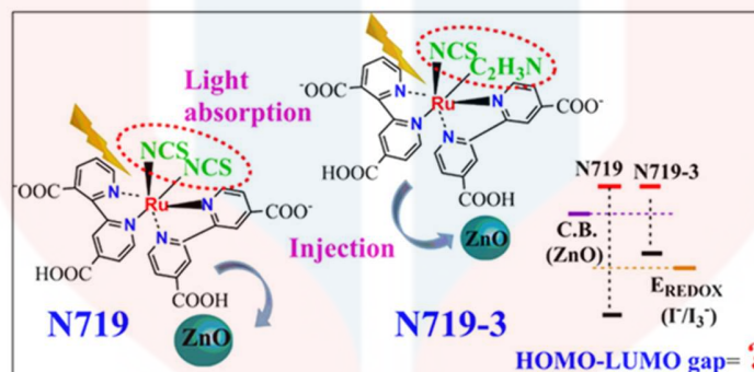
Figure 2.3: N719 Derivatives for Application in a Dye-Sensitized Solar Cell (DSSC) (Portillo-Cortez et al., 2019)
