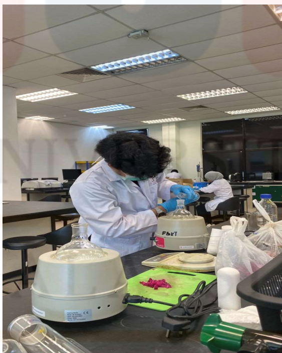
Figure B.2: Preparation of drying, extraction, and condensation of samples.
