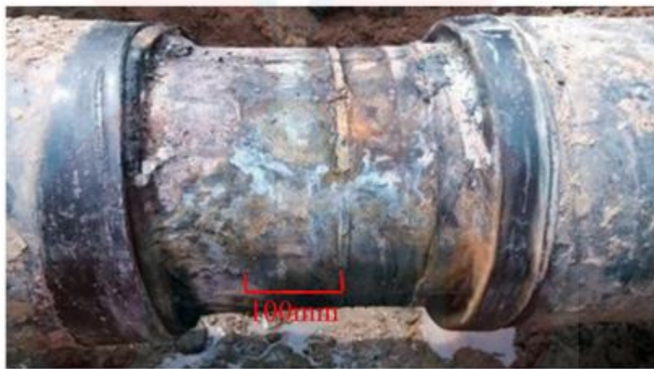
Figure 2.5: Epoxy coating failure
