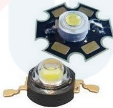
Figure 2.2: Commercial lightning product( Silicone Encapsulation – TIC Industries, n.d. )
