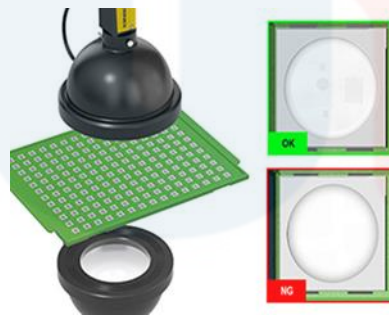
Figure 2.3: High-Power Led encapsulation inspection ( High-Power LED Encapsulation Inspection – Electronics / Cognex, n.d. )
