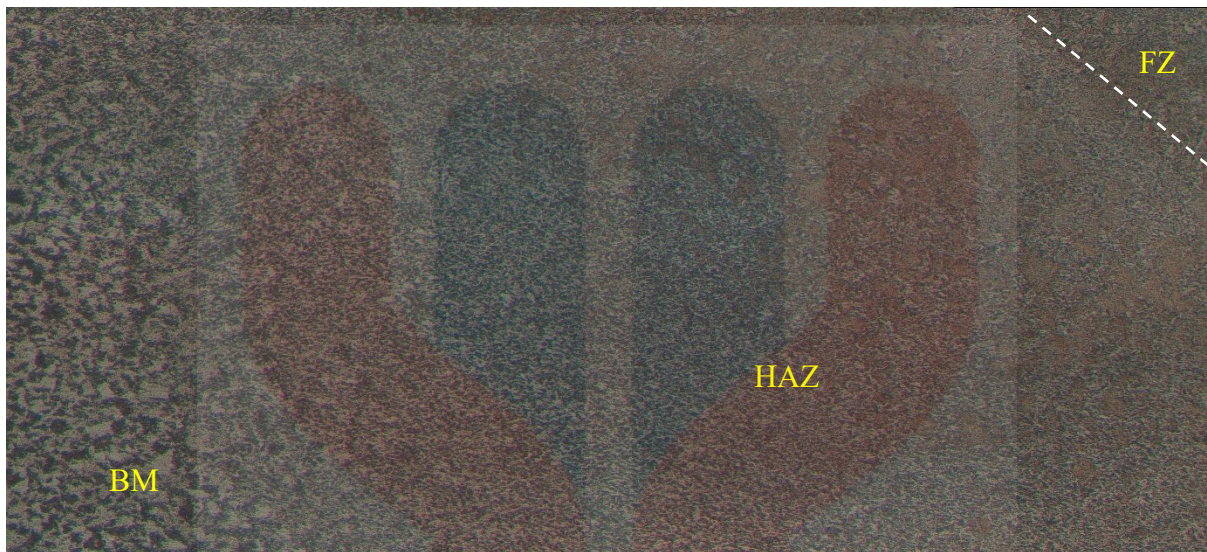
Figure 4. 9: Microstructure of multi v groove in HAZ under 50x magnification
