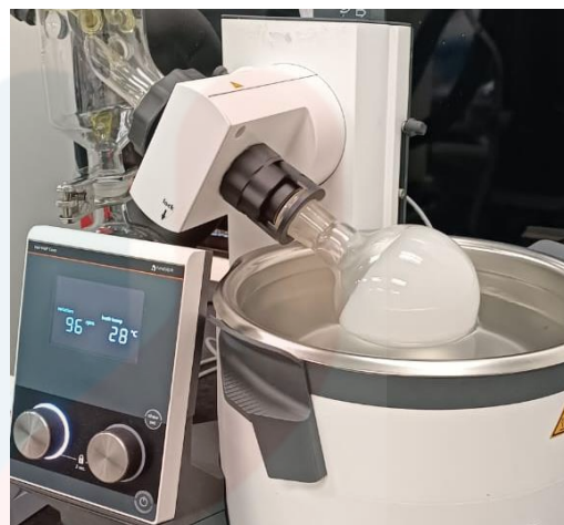
A.2: Solvent evaporation process using rotatory evaporation.
