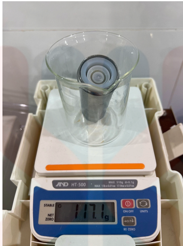
Figure 3 : A compact scale (A&D HT-500) was used for counterbalance.
