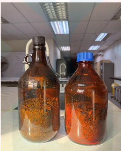
Figure 3.2 Soaked sample in hexane and methanol.
