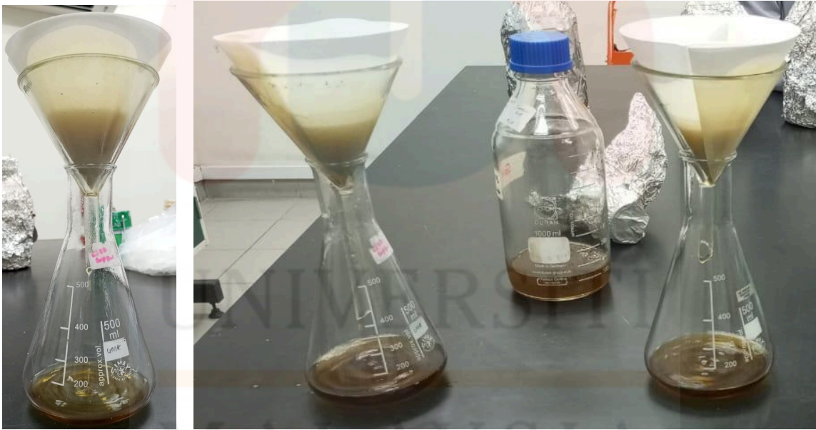
Figure 6 : Filtration process of the soaked plant powder
