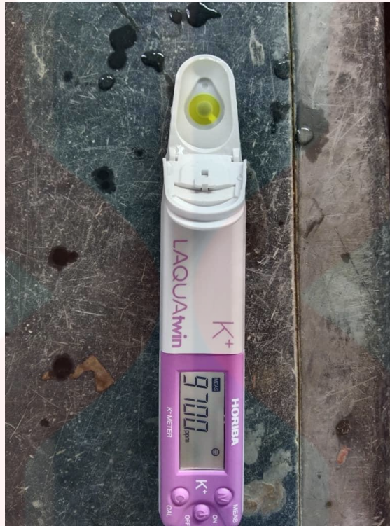
Figure 4.27: Process of identifying potassium content using Horiba LAQUAtwin
