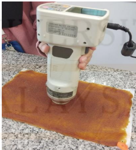
Konica Minolta Chroma Meter CR-400 to observe colour analysis
