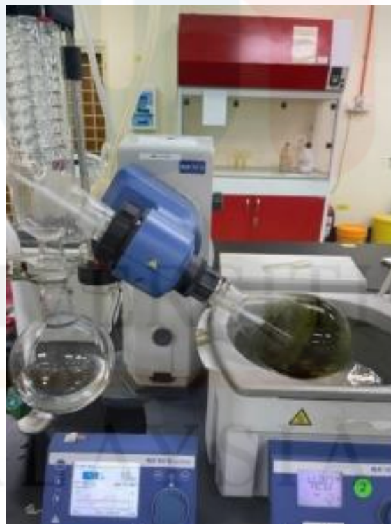
Figure 5: Shows Rotary evaporator used for removal of solvents from samples
