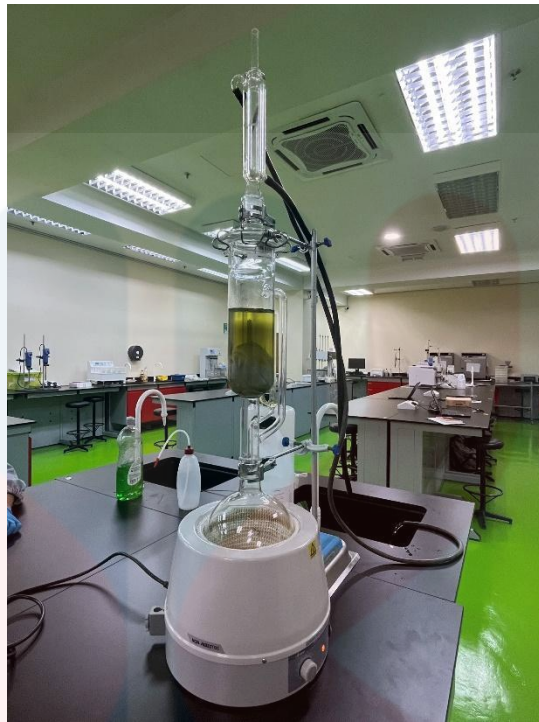
Figure 4: Extraction using Soxhlet apparatus
