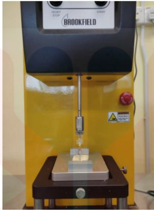
Figure B.8 Texture profile analyzer (Brookfield)
