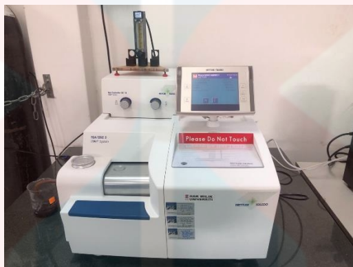
Figure 3.13: Mettler Toledo TGA/DSC 2 GmbH Star System
