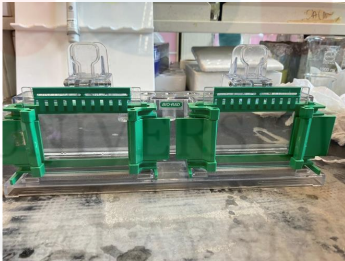
Figure B.8: Using the casting plates to form the gel using the resolving and stacking buffer
