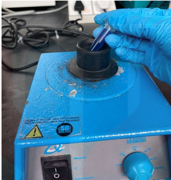
Figure B.3: After centrifuge, put 1000 \mu l of Bradford reagent and vortex it
