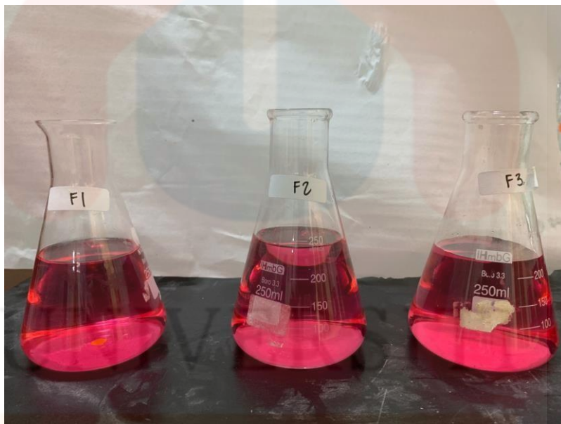
End-product of Kjeldahl titration process of treated rabbit meat
