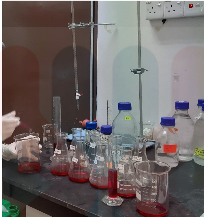
Figure A.11: One of Kjeldahl steps (Preparing the receiver for distillation)
