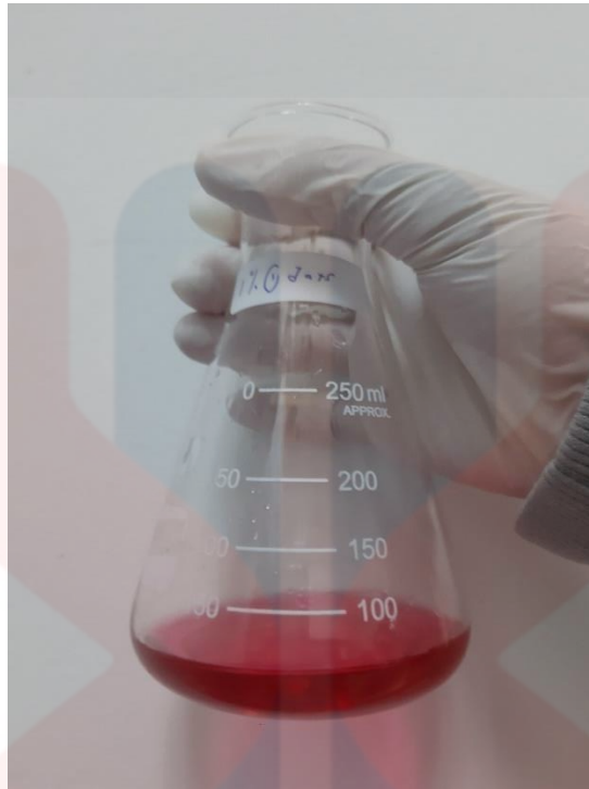
Figure A.13: The pink colour of receiver for distillation in a 250 ml of conical flask
