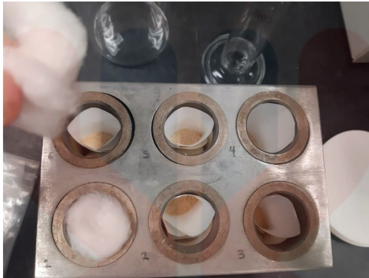
Figure A.19: One of the processes in analysis of fat by using the Soxtec (FOSS) fat analysis machine (Preparing the sample in the thimble)
