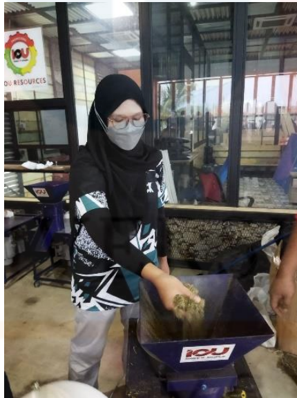
Appendix B.9: The mulberry complete formulation feed were put into pelletizer machine.
