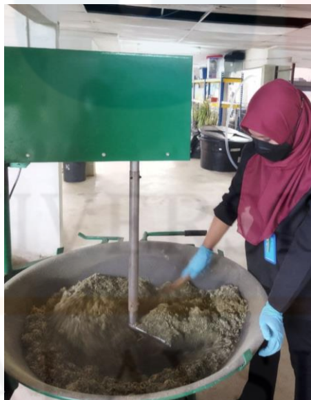
Appendix B.7: The mixing of all raw ingredients using mixer machine.
