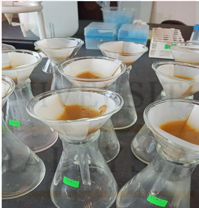
Figure A.2: Filtering the sample soil sample
