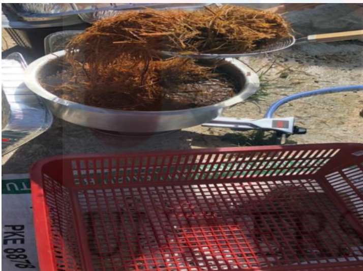
Final step, after 30 minutes boiled, rice straw dried for a while before processes mixing.
