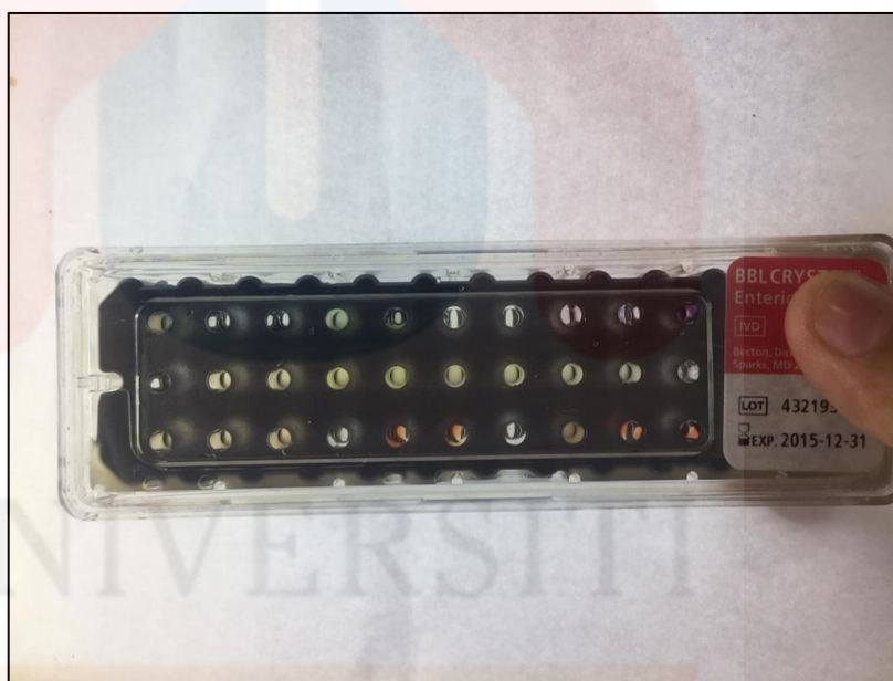
Figure 3.5: BBL Crystal kit for bacteria identification
