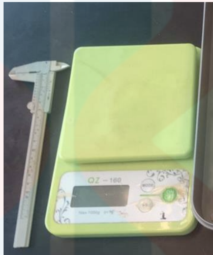
Figure 3.3.1.5: Vernier scale and balance scale
