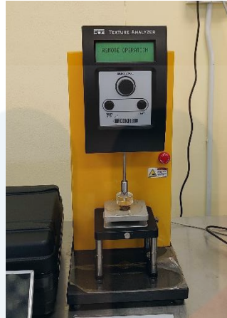
Figure A.7: Textural Profile Analysis (TPA) for hardness, cohesiveness, and springiness by using Brookfield CT3 Texture Analyser with cylinder probe.
