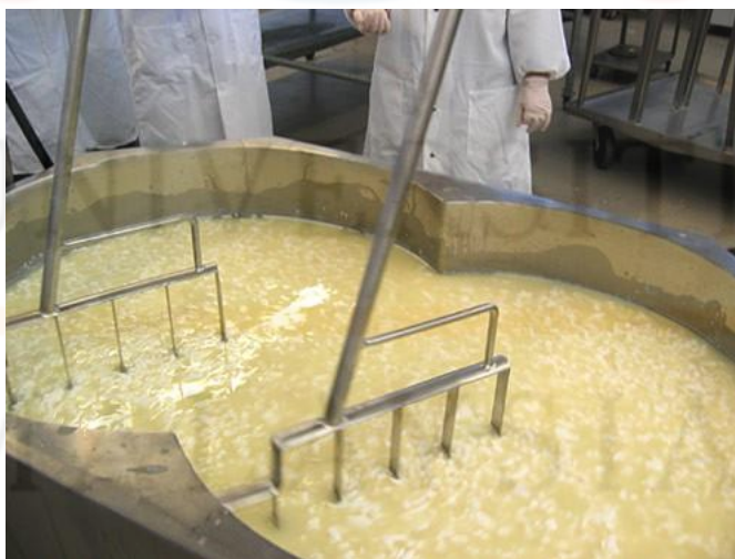
Figure 2.5: Separating curd by using cheese harp (Source: Science buddies, 2021)
