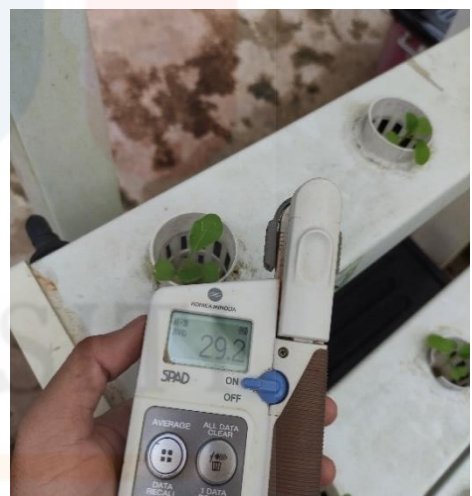
Figure A4 : Measuring Green Mustard Chlorophyll using a SPAD Meter.
