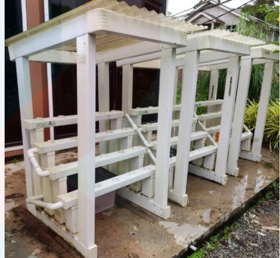
Figure A1: Hydroponic NFT rack used for 3 treatments
