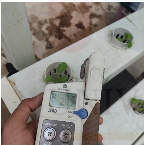
Figure A4 : Measuring Green Mustard Chlorophyll using a SPAD Meter.
