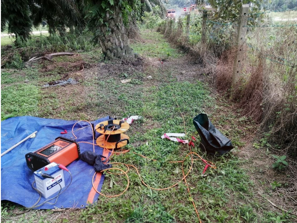
Figure 5.15: Instrument set up of survey line 5. (Source: Dr Hamzah Hussin, 2019)
