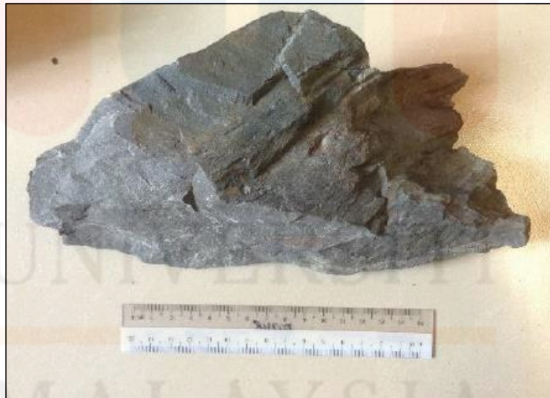
Figure 4.16: Rock sample of shale featuring its fissility (Source: Mohamad Khalim N.S., 2018)
