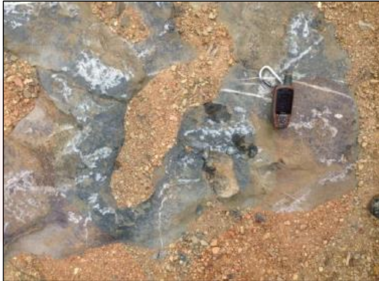
Figure 4.19: Carbonaceous mud limestone discovered in the study area
