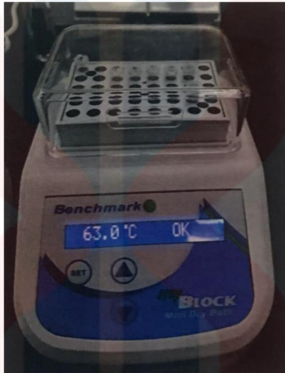
Appendix A: RT-LAMP incubation of extracted oropharynx swab samples from cats using heating block at 63°C
