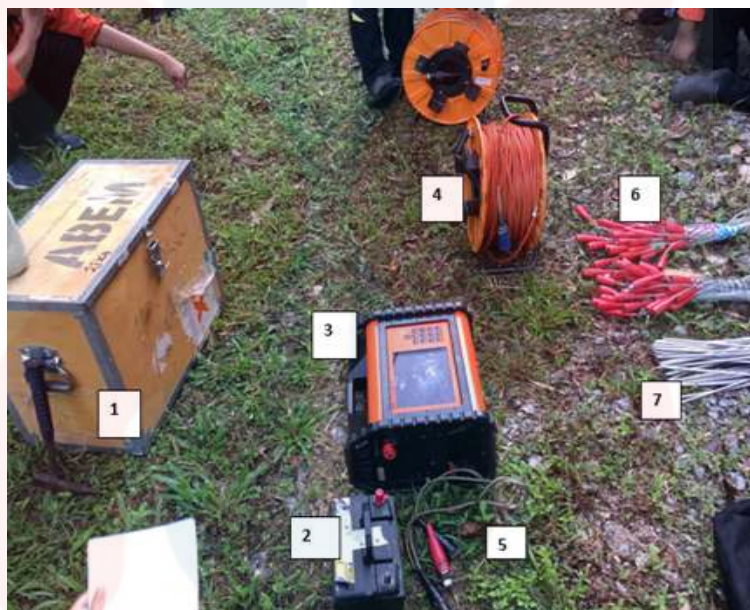
Figure 3.4: Tools for resistivity survey.
