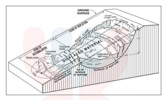
**Figure 1.1**: Terminology for describing landslide features (Cruden & Varnes, 1996).
