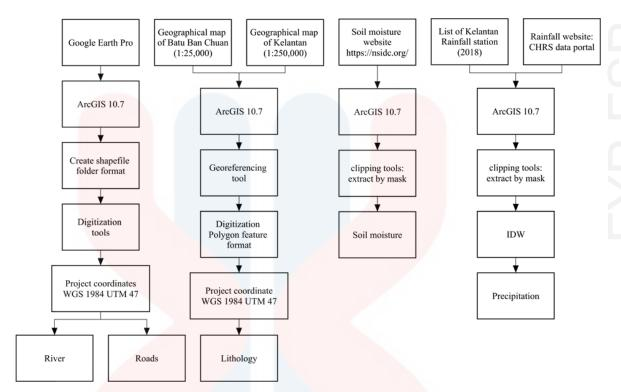
Figure 3.2: Flow chart for the production each of the parameters map
