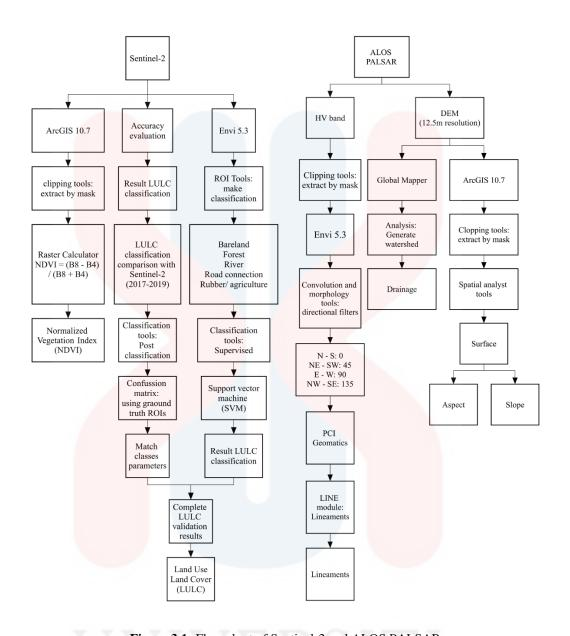
Figure 3.1: Flow chart of Sentinel-2 and ALOS PALSAR
