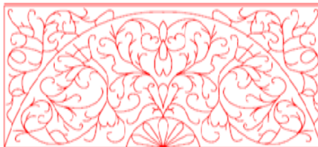
Figure 4.3: Single line CADD of ventilation panel overlapped with 200mm x 200mm grid and produced point pattern.
