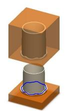
Figure 6: CAD Mould created with Solidworks
