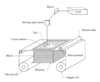
Figure 2: Illustration of the working principles of LOM Source: http://blog.nus.edu.sg/u0804594/files/2011/10/LOM-Process.png
