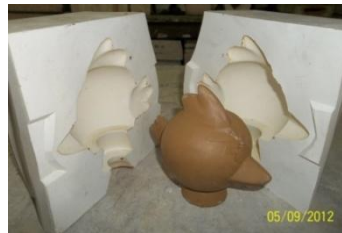
Figure 5: Plaster mould with the casted piece
