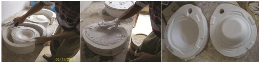
Figure 4b: Pictures illustrating how master mould is created from case mould
