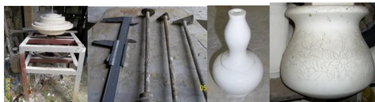
Figure 2: The turning wheel, shaping tools and models created
